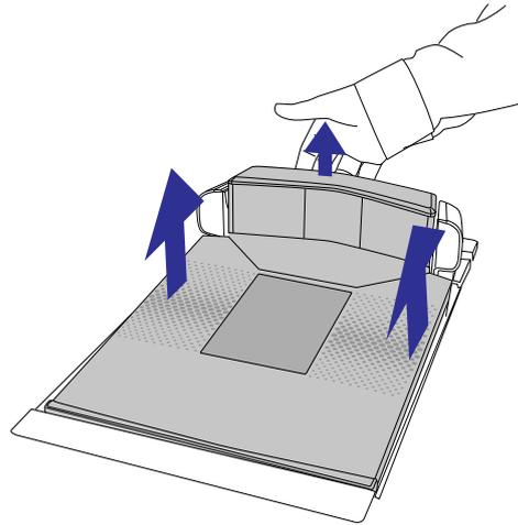
2. The Vertical Scan Windows are held in place by the flat wedge-shaped plastic piece (Figure 5) directly in front of them. To remove it, carefully release the six tabs on the underside of the platter as shown in Figure 5, then carefully turn the platter over and gently lift the plastic piece off of the platter.
