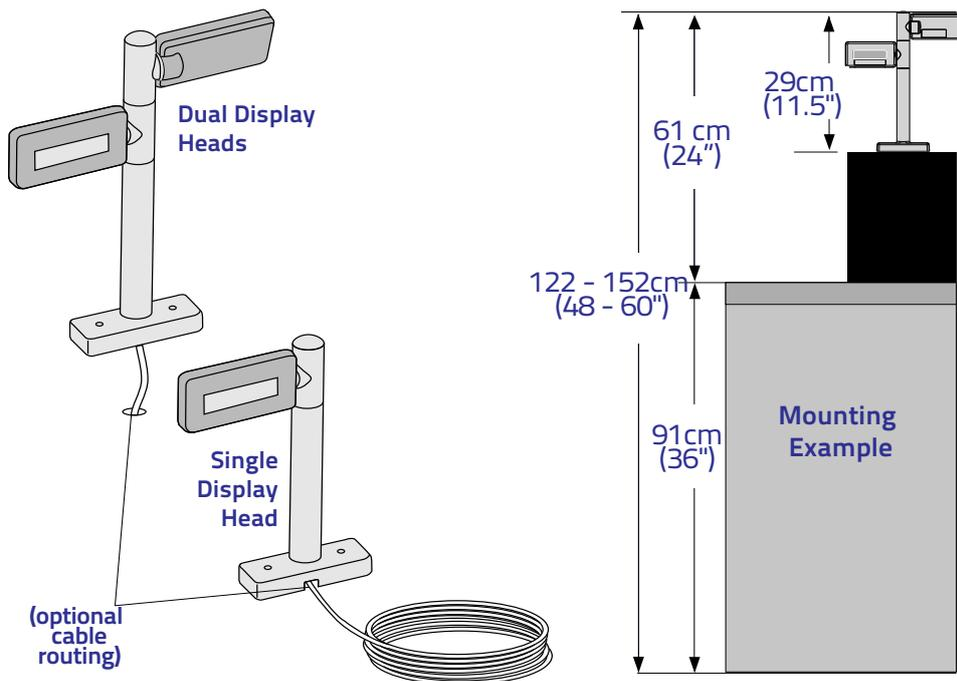
Figure 24. Remote Scale Display Mounting Template
