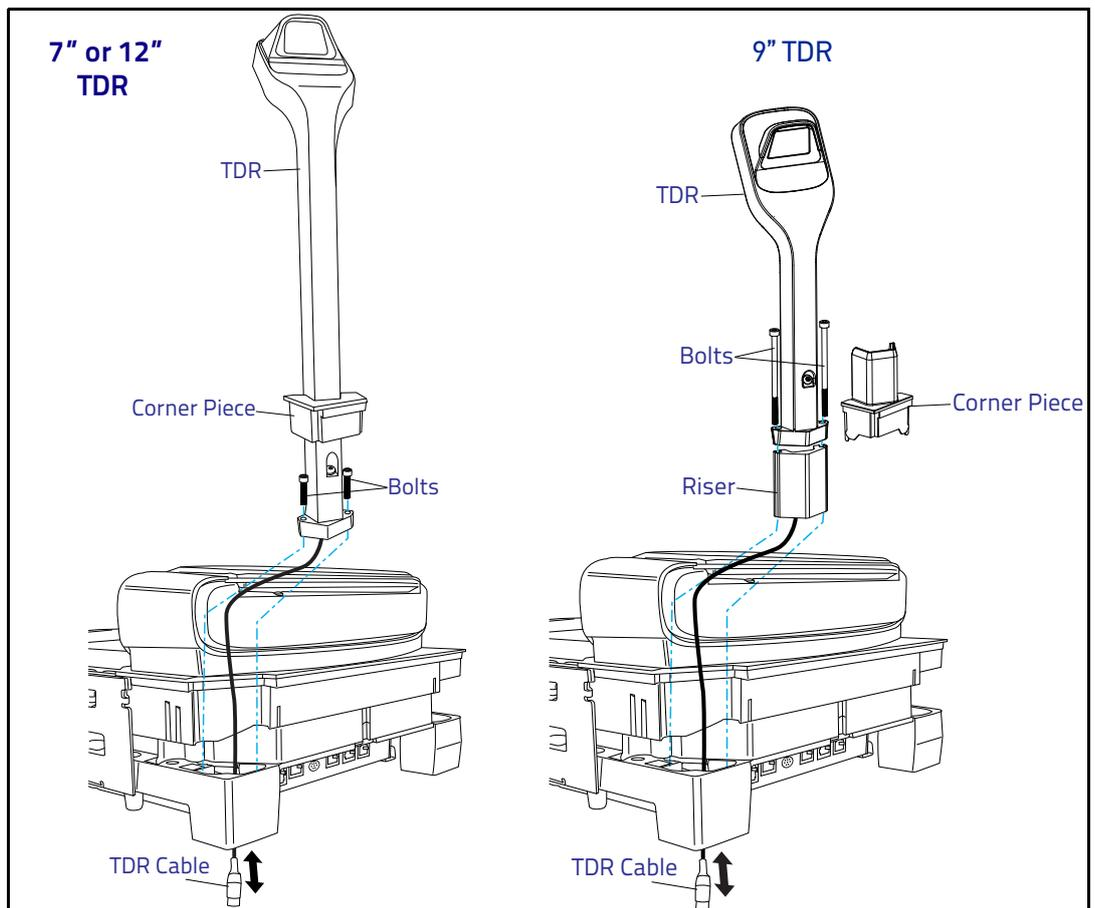
4. [For 9" TDR ONLY]- slide the provided long bolts through both the TDR and the Riser.
