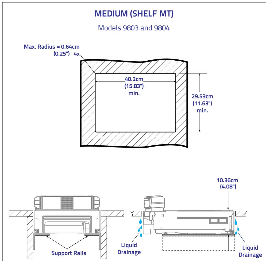
Figure 9. Counter Cutout and Scanner Support Dimensions - Long
