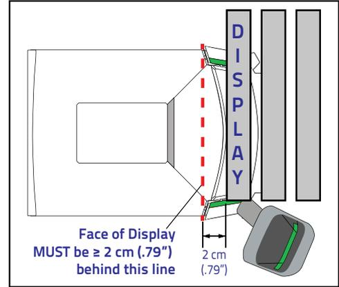
Figure 4. Scanner and Scanner/Scale Models
