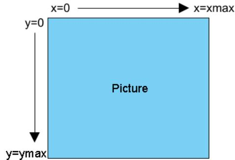
Where **xmax** is the x-size of a full size image (1279 pixels), and **ymin** is the y-size of a full size image (1023 pixels).
