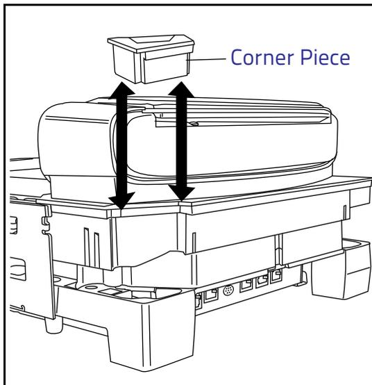
2. For 7" or 12" models, gently slide the Filler Tab from the Corner Piece. This will leave an opening for the neck of the TDR. [For the 9" model, use the new Corner Piece provided.]
