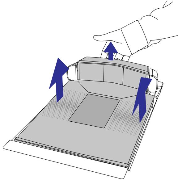
2. The scanner provides lift handles that must be rotated up into position for use as shown in Figure 20. When released, these handles should be allowed to rotate back down into their seated positions in the cavity. Use reasonable care when attempting to lift the unit using any features other than the lift handles.
